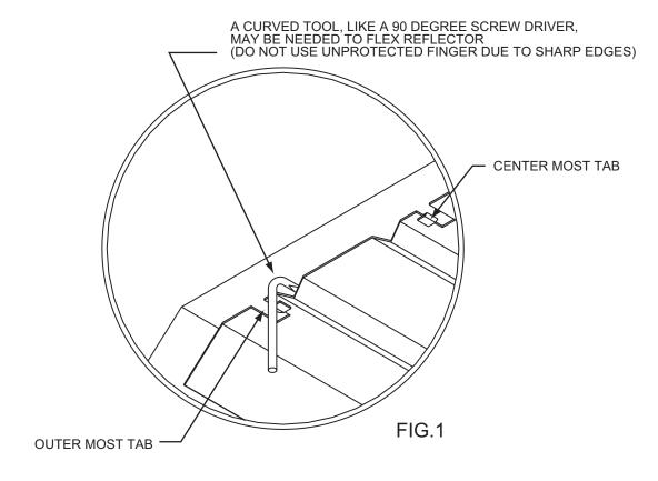
NOTE: WHEN FLEXING REFLECTOR TAKE CARE NOT TO DISTORT REFLECTOR.
